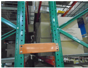
Spacers between rack rows reduce the likelihood of tipping. Wall spacers also help protect the wall from fork damage.
