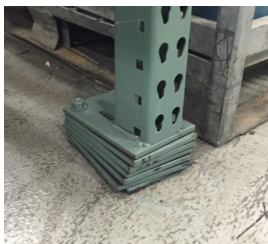
If several shims are needed for leveling, they should be welded together.
